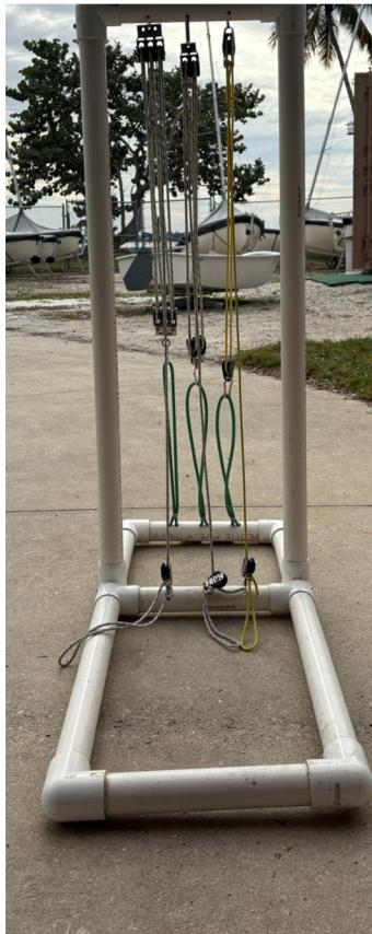
Harken Blockheads and New England Ropes provided 400 feet of line and more than 90 blocks to demonstrate the mechanical advantage of purchase systems.
