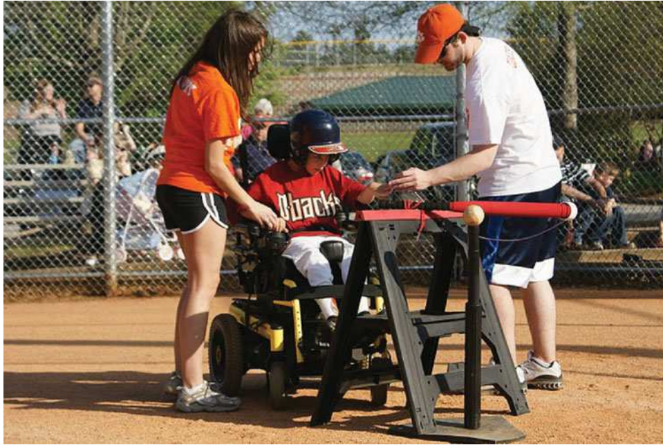
Fig. 1. Batting device that swings when lanyard is pulled by athlete. Photo © Dwayne Fennell (color figure available online).
