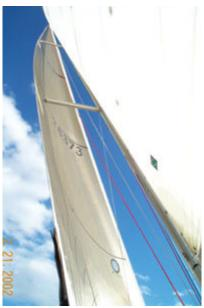
Since the genoa is often pushed up in the wind range to cover 0 – 17 knots of wind it is essential to adjust the lead position and trim of the sail as the wind increases. Here you can see the effects of twist. The lead is back and the sheet eased a bit to allow the upper leech to open as the genoa is used at its openend wind range.
