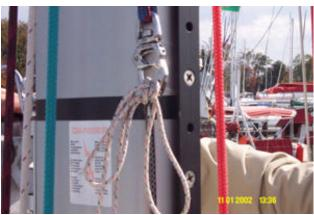
Swing the halyard forward and measure down to the forestay stem/shear intersection. 6' 10 5/8" or 2.10m is what your base setting should be.
