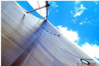
Close sheeting of the genoa is essential due to the long top spreaders of this rig. Once you are at top speed trim until the sail just touches the top spreader. Note the very close rig confirmation of this sail it nearly touches each spreader and the shroud base.
