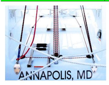
The backstay is an essential control for power, speed, and point. It needs to be played constantly and with each puff. Moving the backstay controls so that the mainsail trimmer can play it constantly is the single biggest improvement you can make to your boat.
