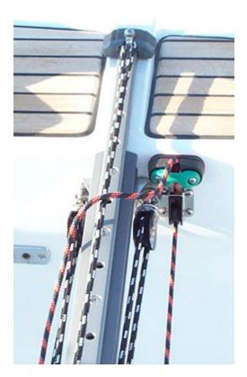
For the mainsail trimmer the standard traveler control is a bit of a rough ride. The trimmer is forced to sit with a double block in his bum; this makes for some interesting bruises. We recommend removing the double block at the end of the track and installing 2 single blocks as shown in the photo. This will please your mainsail trimmer and clean up the deck nicely, it also aids in line management. Note the backstay control line and cleat set next to the traveler.
