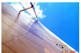
The Blade Jib is designed to be very close sheeting and will trim 6"-8" inside the spreader tips.
