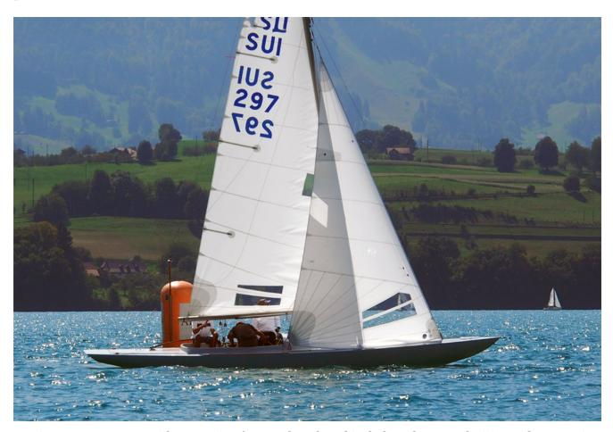
Tuning a Dragon starts with measuring forestay length and includes other complexities such as running backstays and adjustable shrouds that can be tensioned underway. Photo: North Sails Schweiz
