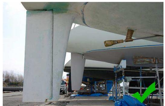
Skeg clearly visible as is propeller
