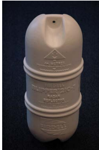
Figure 8 Photo of a Firdell 210-7 reflector
