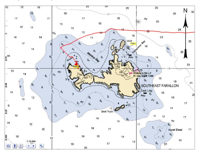
One anomaly with LSC's track is the small northward "kink" shown just north of "North Ldg" on the chart, skirting the 6 fathom depth contour. This appears to be a GPS tracking anomaly, as part of that "kink" is missing GPS data shown by a dashed line.
