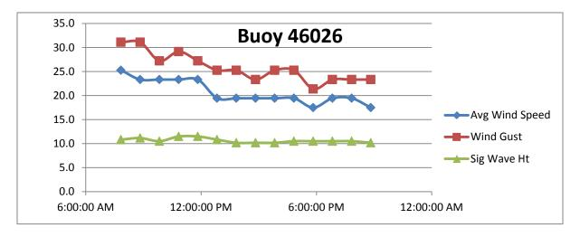
Buoy 46026 is partly sheltered from some waves by Point Reyes. There is also a "Waverider" buoy (46214) 20 miles west of Pt. Reyes and 25 miles NW of the Farallones, in deep water at the edge of the continental shelf. Since this buoy is some distance from the Farallones, consideration needs to be given to how long it takes waves to travel the 25 mile distance.
