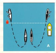
Quite often the boats have to sail backwards out of this position. To enable this, the crew backwind the jib (foresail) onto the opposite side, which pushes the bow of the boat around.
