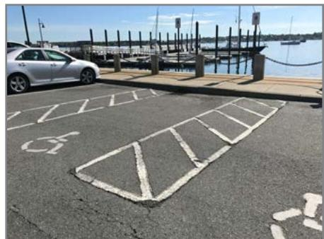
Parking should be close to the building, dock or beach and have enough space for a car door to open completely, or for a van to lower a ramp (approximately 8 feet). Clear signage for designated spaces reserved for drivers and passengers with disabilities should be installed.
