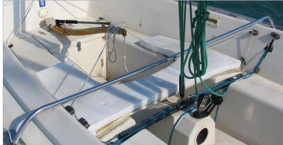
Often, a transfer bench is used in conjunction with a grab bar so the sailor can use upper body strength to transfer while the boat is heeling. If a grab bar isn't available, tie a length of thick line (at least  $\frac{1}{2}$  inch in diameter) from one side of the boat to the other and tension tightly to provide some stability during the side-to-side transfer.
