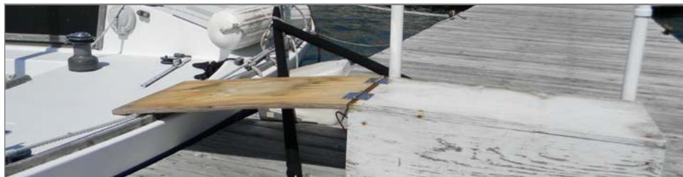
A transfer board allows the sailor to transfer directly from their chair to the boat by sliding from one to the other. Sailors with vision impairments may also find transferring via a board or box easier than stepping over the side of a boat, especially if there is a large gap.
